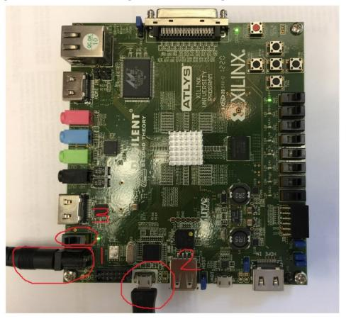
Plug in the power cord, then the usb cable from the board to the computer, and finally turn on the power switch.
