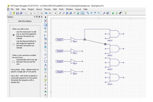
To add a wire to the schematic, either click on two different points or drag the wire from one point to another. These points can either be a blank space, one of the tiny blocks connected to each symbol, or another wire.
