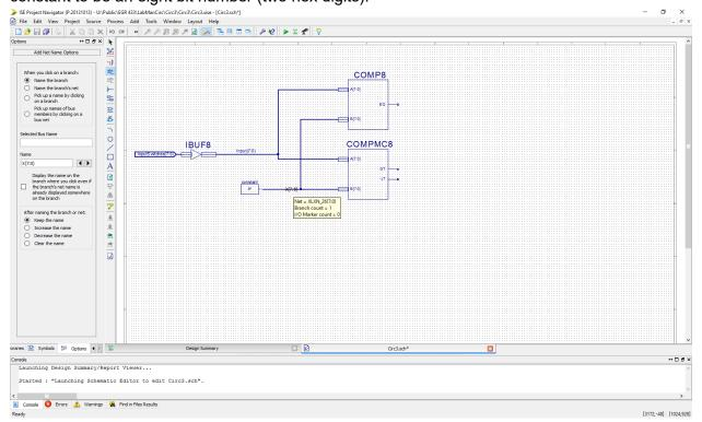
Attach the constant to the second input in each of the comparators.
