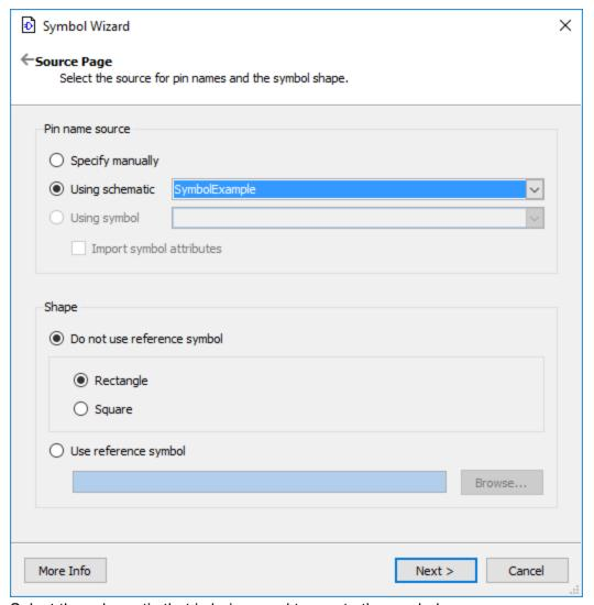
Select the schematic that is being used to create the symbol.
