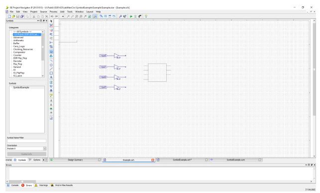
You can locate the created symbols under the file location that the schematic was in in the add symbols section of Xilinx. Add the symbol to the main schematic.
