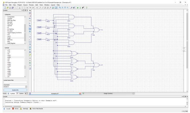
Next, we are going to add a symbol that tells us when it is a tie (neither of the four-input OR gates have a value of 1). Instead of using a two-input NOR gate, let's use the and2b2 gate. To figure out what it is, click on the name of the symbol and then click Symbol Info. Place it on the schematic and wire both OR gates to it.
