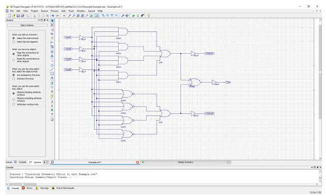
Connect three output markers received from the same location as the input markers on the right side of each output buffer. This is what the completed circuit should look like.
