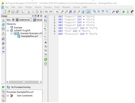
The final step is to create the implementation constraints file and state where the inputs and outputs are to be located on the FGPA. You are now done with the first example circuits.
