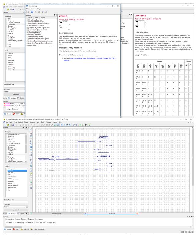
There are two different comparators in Xilinx, one that says whether or not they are equal and one that says whether the first input is greater than or less than the second. We will be using
