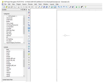
Under the IO Components, select the input buffer (ibuf). Place four of them on the schematic.
