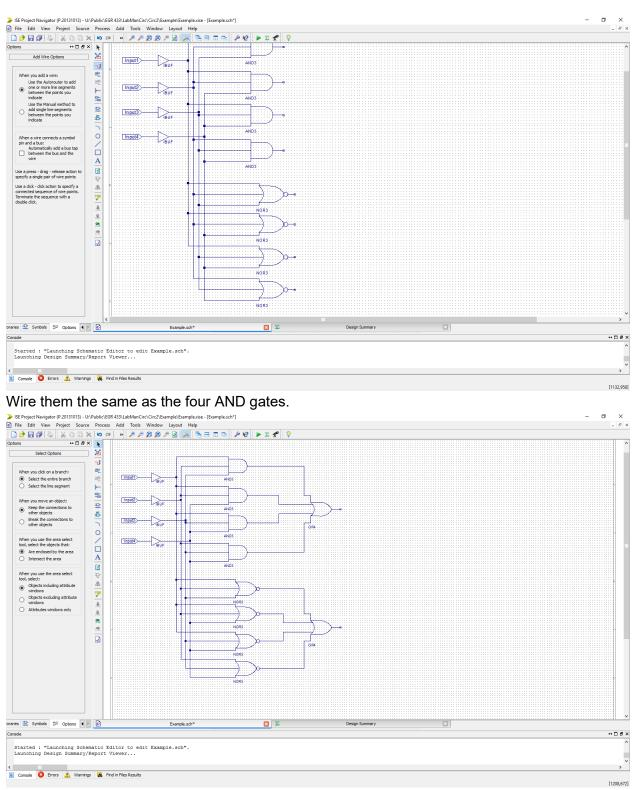
Add two four-input OR gates (or4) and wire each of the AND gates to one and each of the NOR gates to the other.
