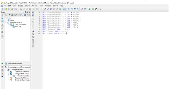
Finally, create the implementation constraints file add state where each of the pins are located.
