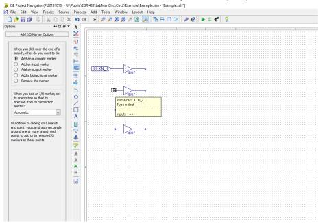
Click on the above icon to access the I/O markers. Put an input marker (or an automatic) on the left side of each of the input buffers.
