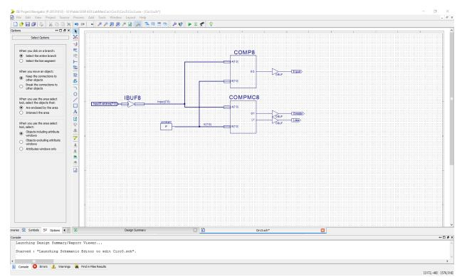
Add output buffers and output markers to each of the outputs from the comparators.
