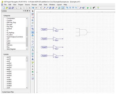
Next, go back to the icon to add symbols, but this time go to logic. Click on the three-input AND gate (and3) put four of them on the schematic.
