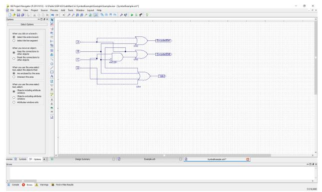
Create the circuit above (an encoder) and add output markers to each of the outputs. Once again, it is important to note that you should not use output buffers in the symbol schematic.
