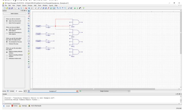
If you do not like how Xilinx automatically placed the wire, you can change its position by clicking on the wire and dragging it.
