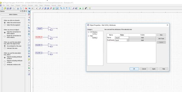
You can double click on the input markers to change their name. To do so, go to the XLIN\_2 under Nets and type the desired name in the name field.
